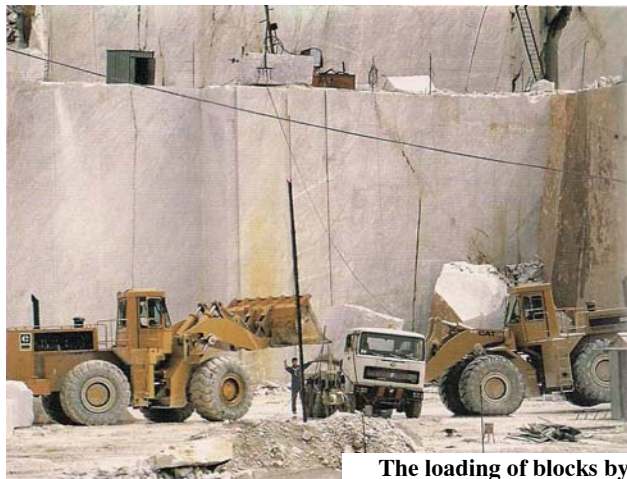
The loading of blocks by means of two scrapers
